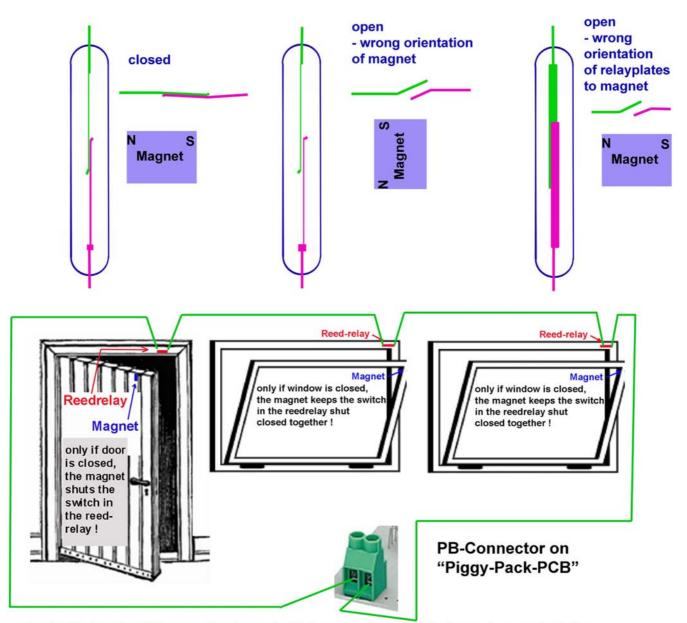
single "intrusion"-loop wired - only if door and both windows keep shut the "wired loop" with all reed-relays behave as a closed line of switches! If only one of the devices gets opened the line becomes "disturbed" i.e. the line is truncared and open and can become detected by the software. Similar other detectors like infrared-detector or shock-detector could also be integrated into this line.
